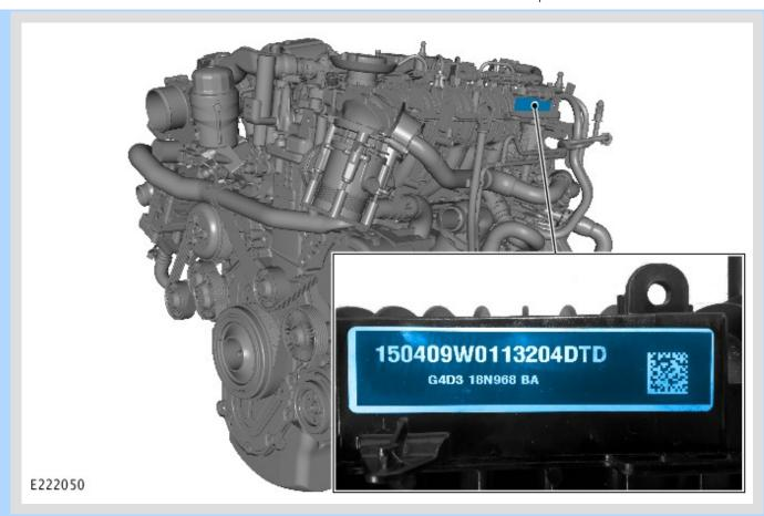
Locate and record the engine serial number.
