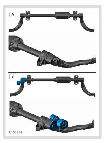
**2013MY Range Rover (L405) vehicles up to VIN 125193 only:** if the knocking noise is still present and considered unacceptable after performing the above steps, replace the Dynamic Response front actuator with part number LR052058 **(B)** (see TOPIx Workshop Manual section 204-06: Ride and Handling Optimisation - Front Stabilizer Bar).
