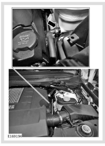
Check the Dynamic Response system fluid reservoir for leaks:
