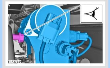
Check the valve block to body stud clearance.
