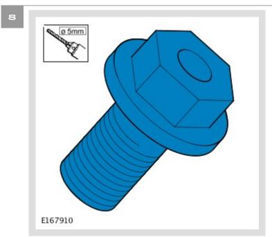
Remove the plastic body fastener and drill an axial hole 5mm diameter through the head; this will allow the body stud to pass through the head of the fixing.
