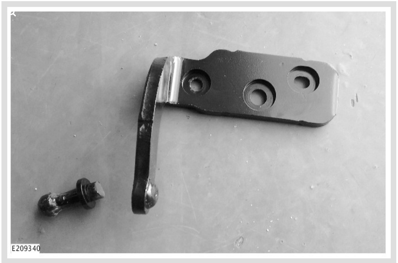
Example: deployable luggage compartment floor operating arm damage.
