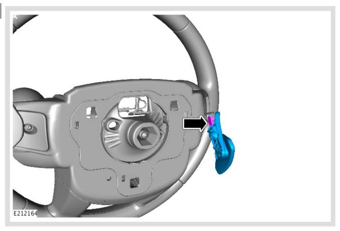
Disconnect the steering wheel left paddle shifter electrical connector.
