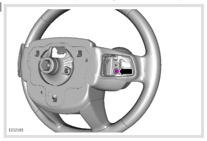
Remove the steering wheel left control switch fastener.
