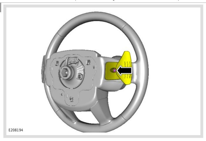
Remove the steering wheel left paddle shifter fastener.
