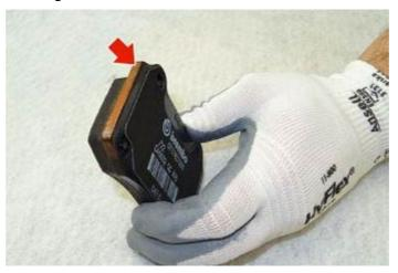
• Rear pads for "Small" system. Smear both pad sides with grease as shown in the figure below.
