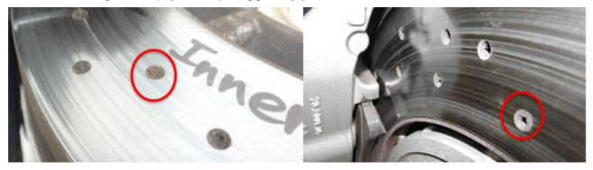
D. Presence of cracks on disc surface.
