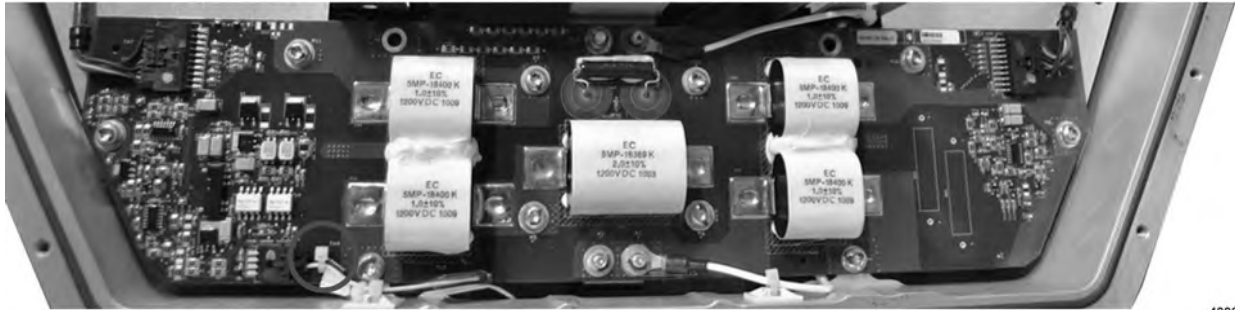
Figure 90. HVIL Circuit Card – Zip Tie Location
