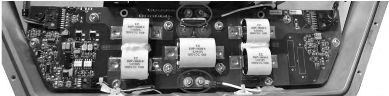
Figure 93. HVIL Circuit Card – Four (4) Mounting Nut/Washer Locations (M5)
