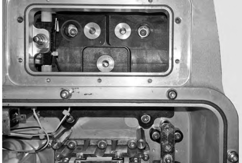
Figure 25. Location of Two (2) M5x22mm Screws
