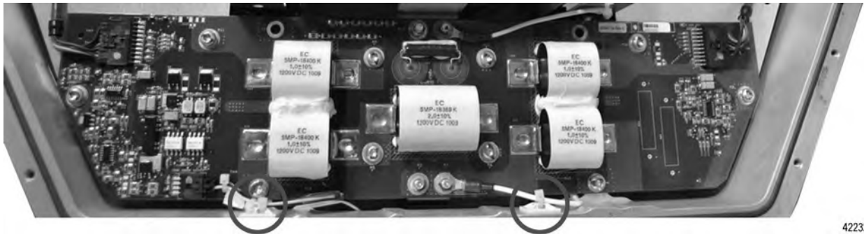
Figure 94. HVIL Circuit Card – Two (2) Zip Tie Locations
