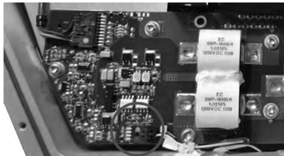
Figure 91. HVIL Circuit Card – Three (3) Harness Connector Locations
