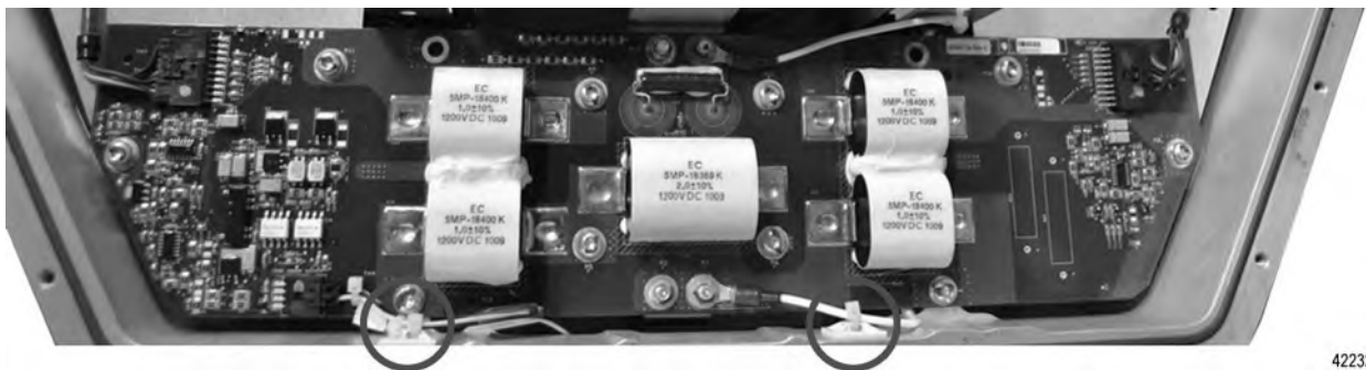
Figure 5. HVIL Circuit Card – Two (2) Zip Tie Locations
