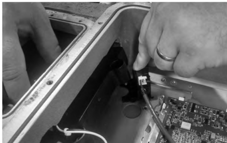
Figure 36. Installation of Current Sensor
