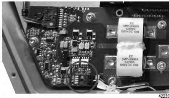
Figure 7. HVIL Circuit Card – Three (3) Harness Connector Locations
