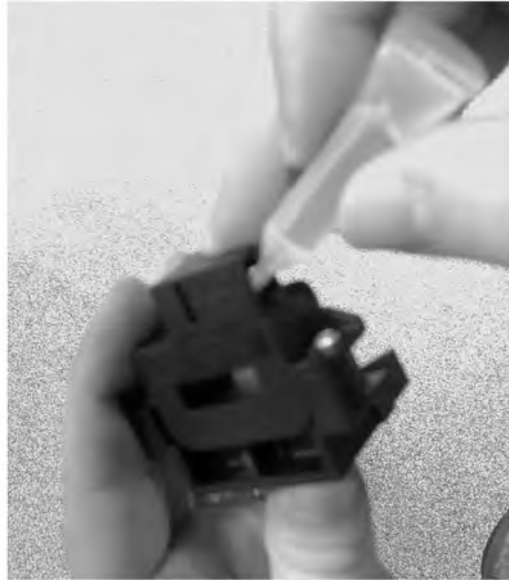
Figure 35. Applying NyoGel® 760G lubricant to Current Sensor Pins
