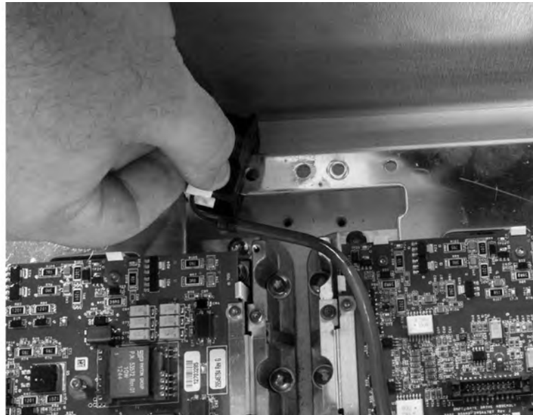
Figure 51. Removal of Current Sensor
