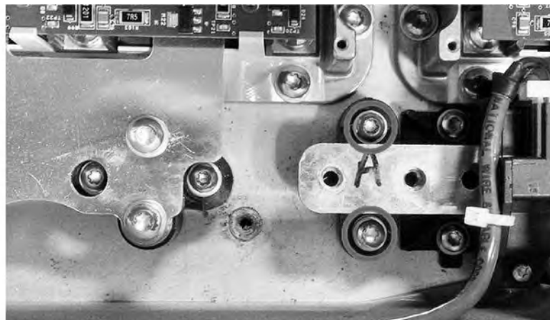
Figure 59. Location of Two (2) M4x22mm Screws
