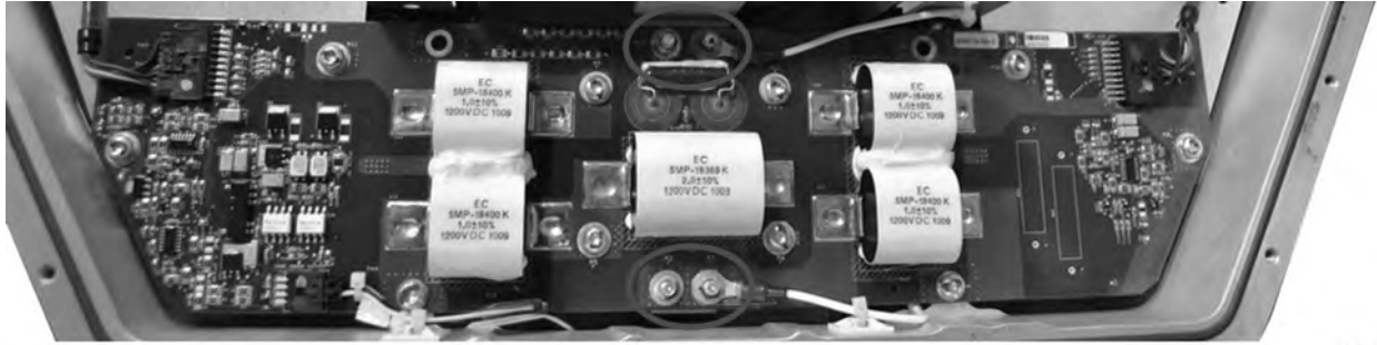
Figure 8. HVIL Circuit Card – Four (4) Mounting Nut/Washer Locations (M5)
