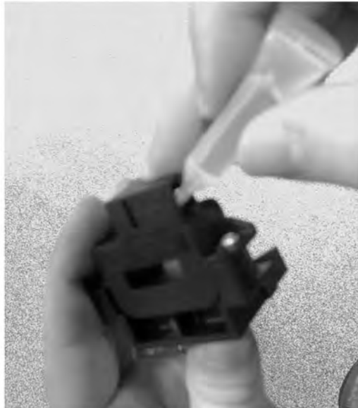
Figure 53. Applying NyoGel® 760G lubricant to Current Sensor Pins
