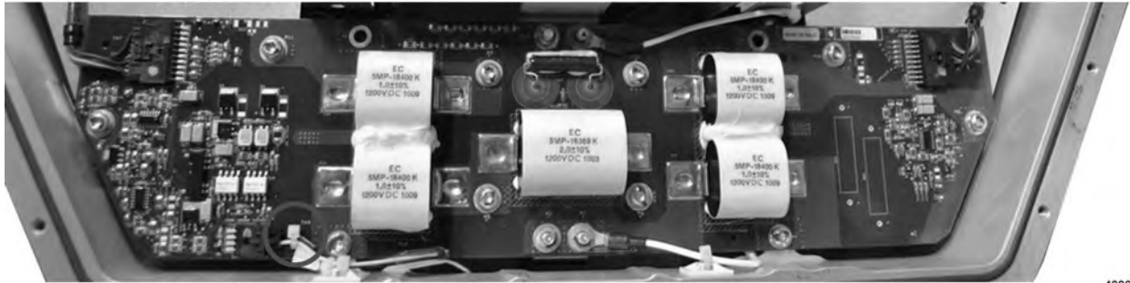
Figure 4. HVIL Circuit Card – Zip Tie Location
