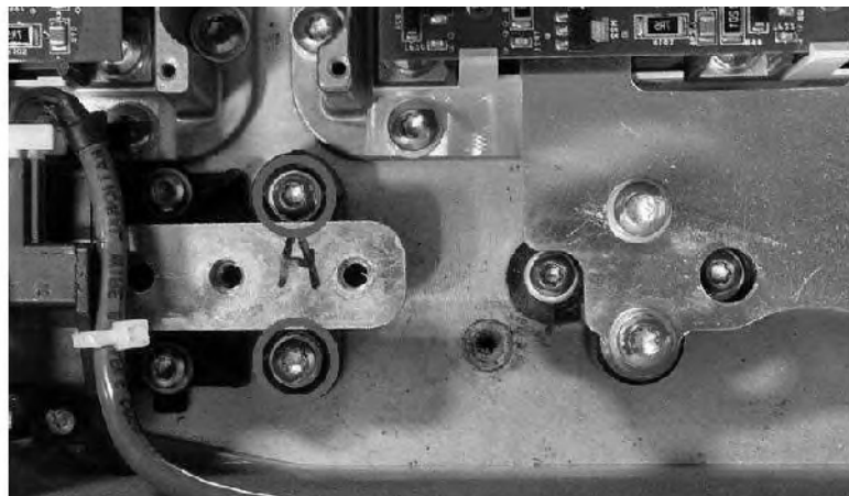
Figure 76. Location of Two (2) M4x22mm Screws
