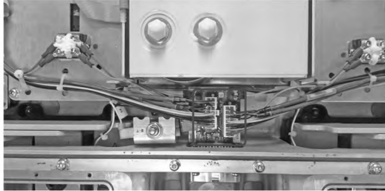
Figure 88. Wire Harness Connector Installation
