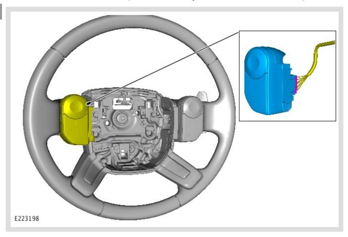
Remove and discard the steering wheel left control switch.
