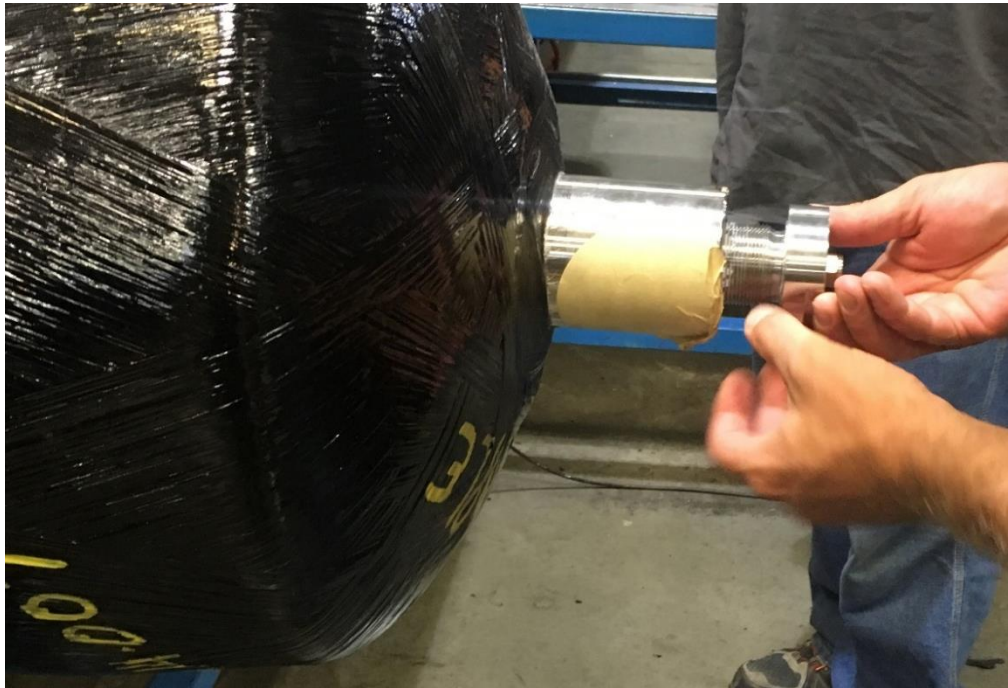
Figure 2. Remove the leaking component.
