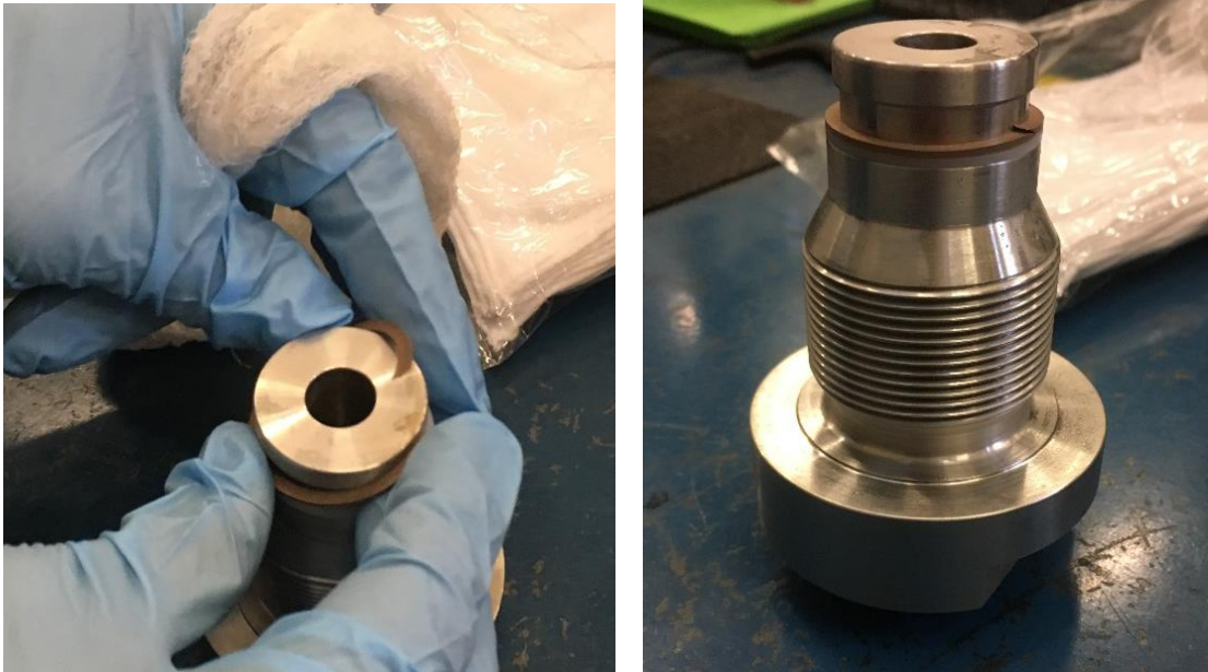
Figure 4. Clean the fitting and install the first seal (backup ring).
