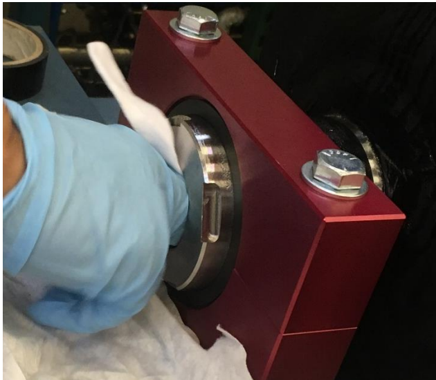
Figure 3. Clean the mating surfaces and install the component.
