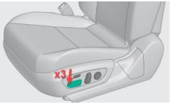
c) Within 10 seconds of (b), simultaneously raise and recline the seat. Hold for about 10 seconds until you hear a beep.
