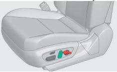
f) Lower the seat all the way down and continue to hold for an additional second.
