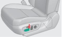
g) Tilt the front of seat cushion all the way down and continue to hold for an additional second.
