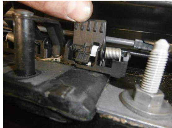
Figure 2. Debris trapped in the rear lid closed sensor.
