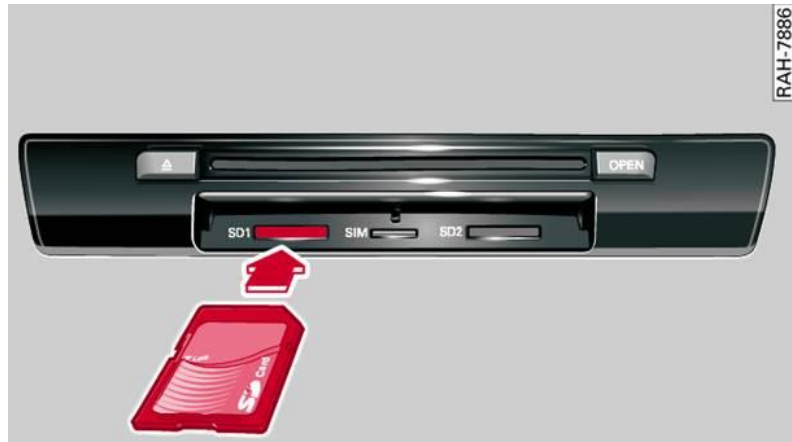
Figure 1. Infotainment control unit (example) position of the SD card for the update.
