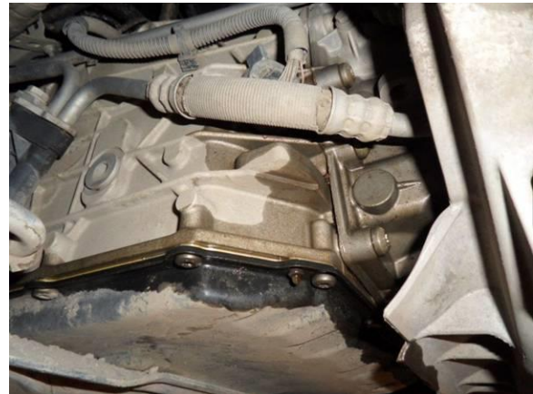
Figure 3. Leak between gearbox housing and intermediate housing.
