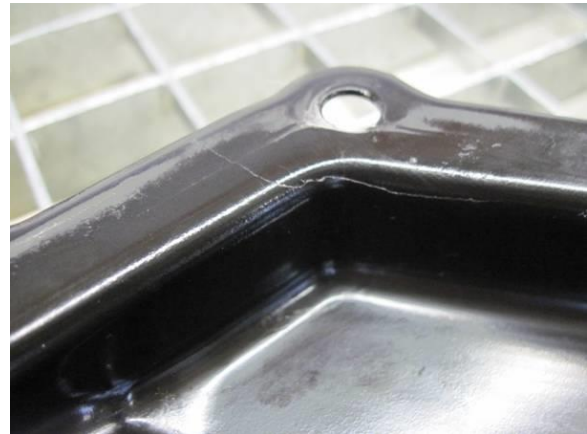
Figure 2. Crack in the oil pan.
