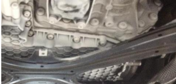
Figure 2: Transmission with oil leak detection spray applied.
