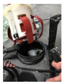
**Figure 1.** Filter element housing loose inside tank.
