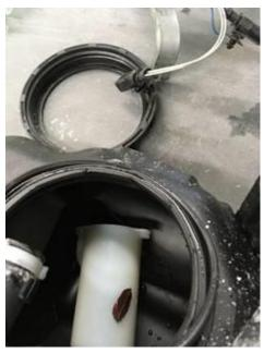
Figure 2. Filter element housing loose inside tank.
