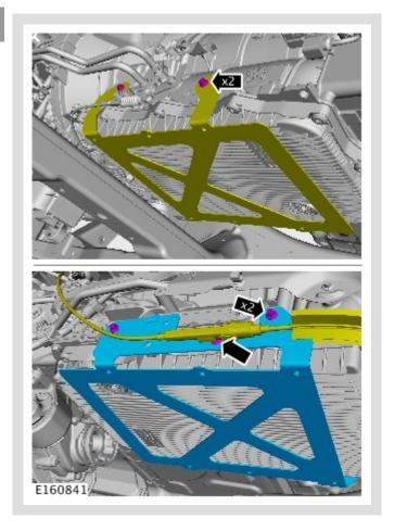
Install the transmission heatshield mounting bracket.
