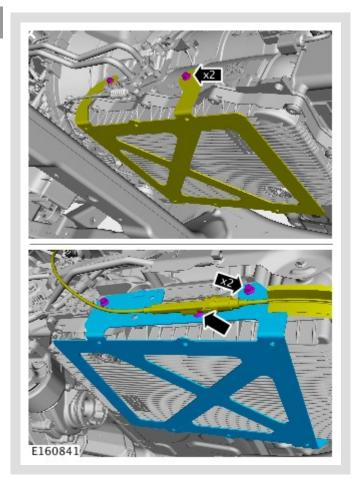
Remove and discard the transmission heatshield mounting bracket.
