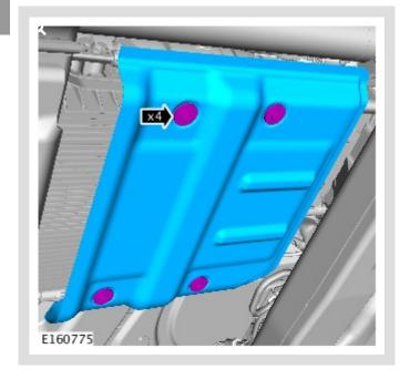
Remove the transmission heatshield.
