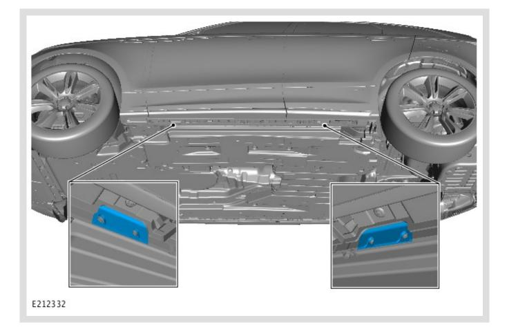
Location of the deployable side step mounting holes.
