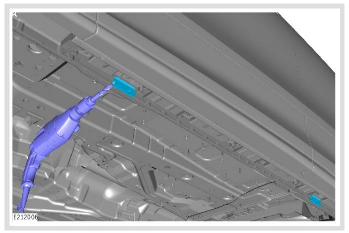
Use an 8.5 mm drill bit to modify the existing deployable side step mounting holes to align the holes.
