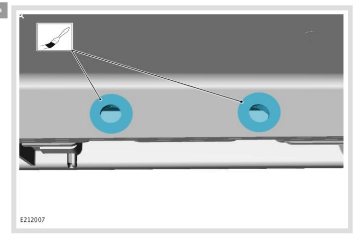
Apply locally sourced Rust-Oleum V2100 System Black Enamel Spray Paint to both sides of the mounting holes.
