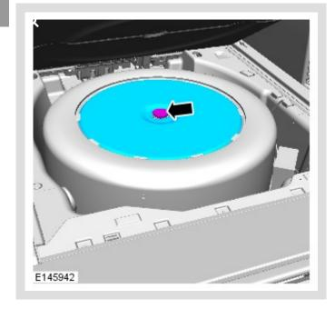
Remove the spare wheel retaining fixing and cover.
