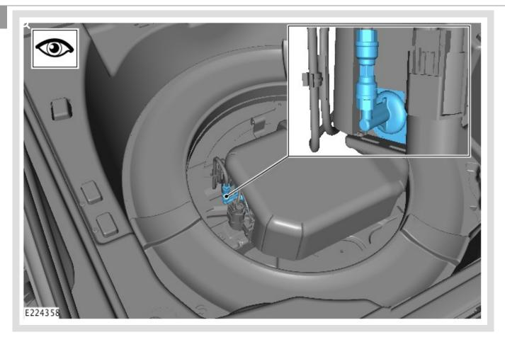
Inspect the suspension air supply unit expansion chamber for damage in the area shown.
