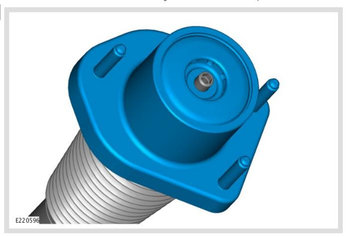
Remove the rear left shock absorber top mount.
