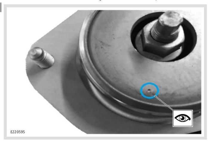
The new top mount should be identified with a 'dot' punch mark on the top plate.
