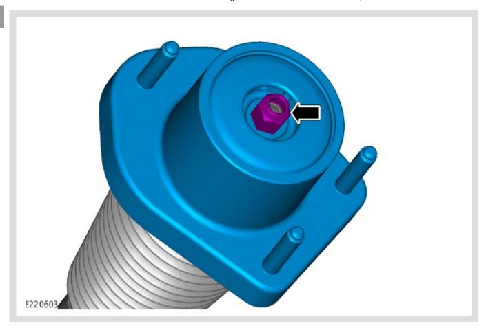
Install the new rear left shock absorber top mount.
