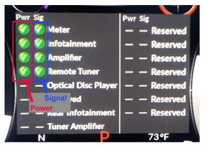
The **Pwr** (Power) and **Sig** (Signal) columns give you the status of each listed component. Each column can have a green check, a red X, or a dash if the component doesn't apply. Here are the possible combinations and what they mean.
