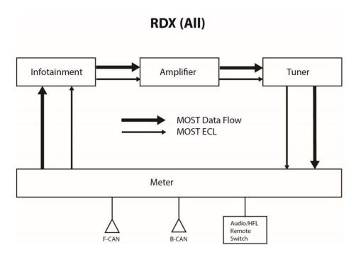
3. Starting with **Meter** on the screen, mark the matching component on your chart with a check mark if communication is good or an **X** if there's an issue. Then, do the same for the rest of the listed components on the screen.
