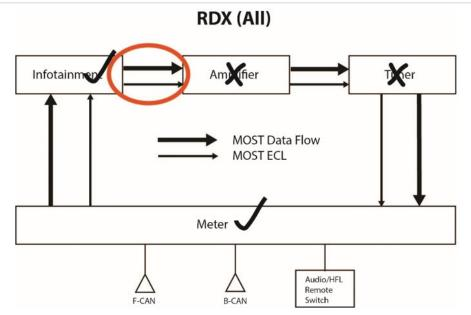
What this is telling you is the problem is either in the connection between the infotainment control unit and the amplifier, or it's an internal fault of the amplifier receiver or the infotainment transmitter. From here, you would check your connections and swap known-good components.
