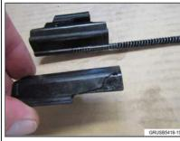
3. If broken sunroof drive components are found, replace both drive cable mechanisms following repair instructions REP 54 13 200 "Replacing drive cable".
