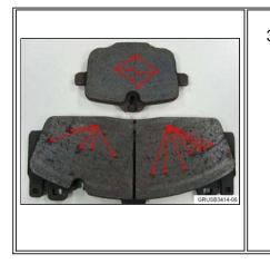
3. After high brake loads, running noises can be heard when applying the brakes, and may also be heard to a limited extent after the brakes are released. (See the note in the Owner's Manual).
