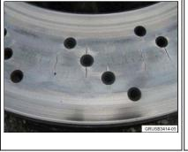
Visible cracks are caused by high thermal stresses during rapid heating and cooling of the brake discs. Braking from high speed with cold brake components (less than 212 degrees F) increases the likelihood of cracks to form. These surface hairline cracks are usually spread over the entire brake disc friction area, and have no negative influence on the durability or braking performance. The rotors should not be replaced only for their appearance reasons.
