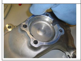
5. Using the part of the cloth containing the lubricant, rub the wheel bearing contact face, thoroughly working the lubricant into the fine scorings created during sanding.
