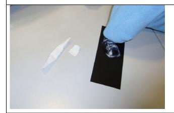
4. Rub all of the lubricant mixture into the tip of a folded cloth.
