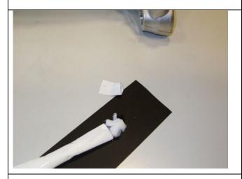
3. Squeeze the components of the provided lubricant onto a mixing surface and thoroughly blend together.
