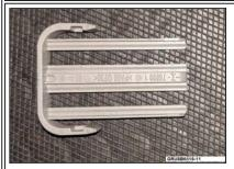
The lock on only one side needs to be removed. This is the lock for the small pin side of the connector.
