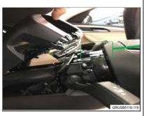
Disassemble the upper steering column shroud, following repair instructions REP 32 31 004 "Removing and installing/replacing steering column shroud upper section".
