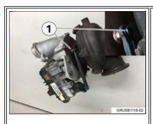
The clips that hold the boost actuator rod for the variable nozzle technology (VNT) turbo have come loose (1).
