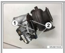
Replace the rod (1) and clips (2) on the VNT actuator/turbo. NOTE: Turbo removed for clarity. The turbo does not need to be removed to complete repairs.
