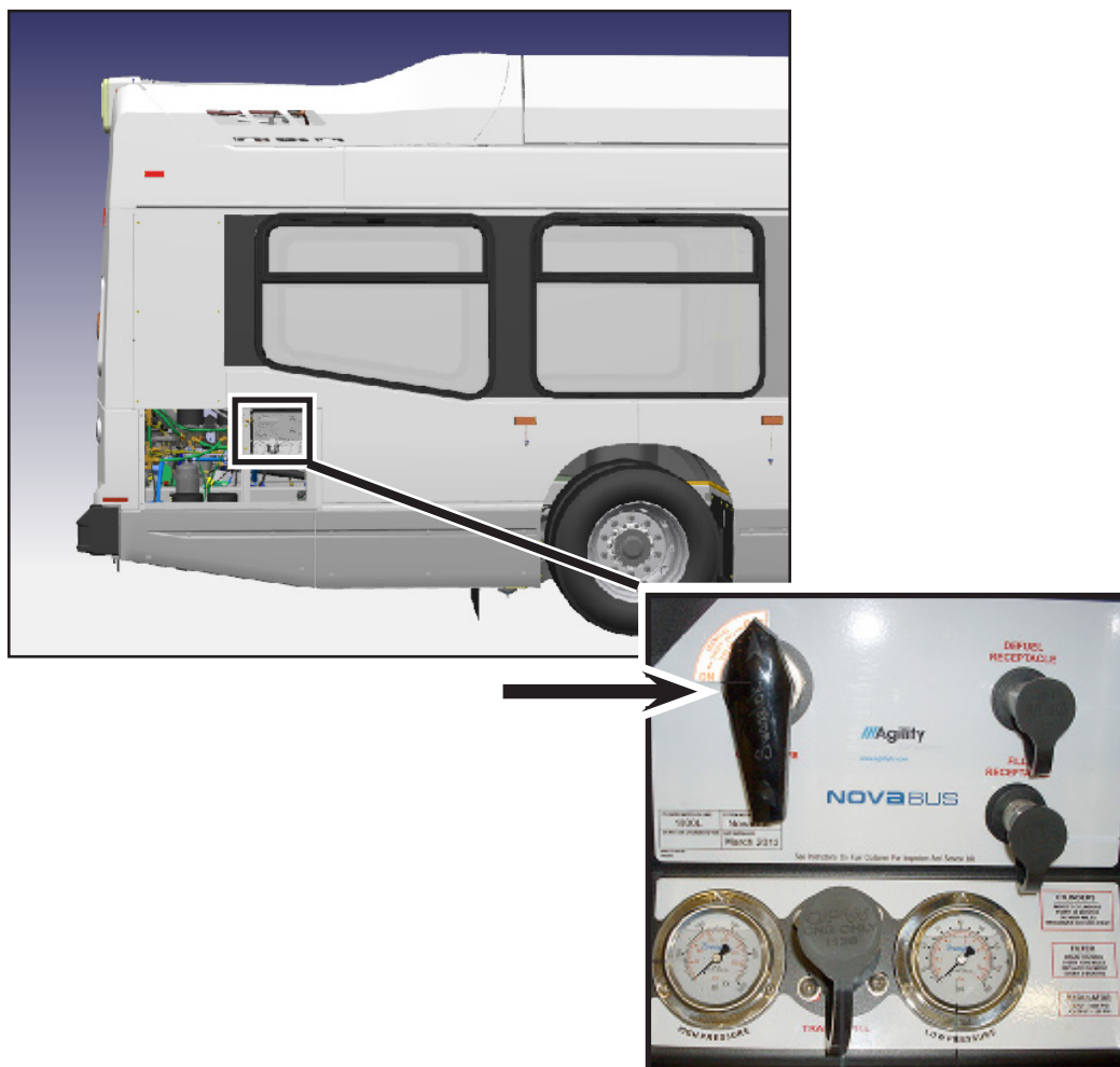
Figure 1 - Shut-off Valve on the FMM
