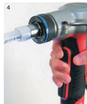
Expansion with Milwaukee M12 ProPEX Expansion Tool
