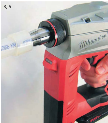
Expansion with Milwaukee M18 ProPEX Expansion Tool
