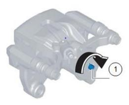
**NOTE:** The procedure on MGSS instructs you to rotate the spindle approx. 2-3 times, which is incorrect for the models specified in this TSB.
