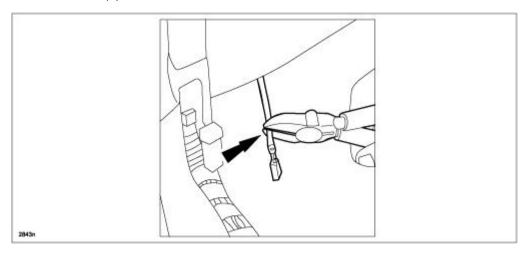
21. Strip 20mm of insulation from the ends of both wires.
