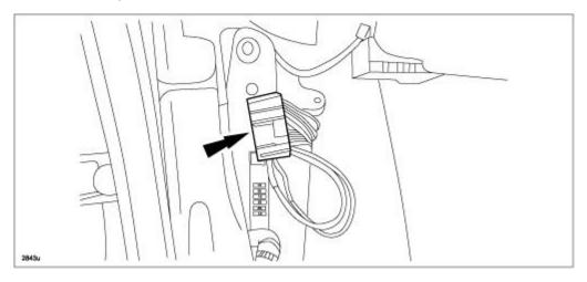
30. Bend the excess length of wires (as shown below) to match with the other wires.
