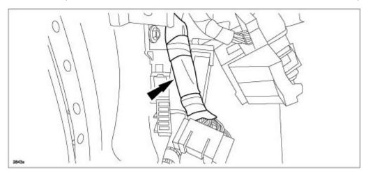
33. Pull out the C-15 connector from the front pillar to the door side.
