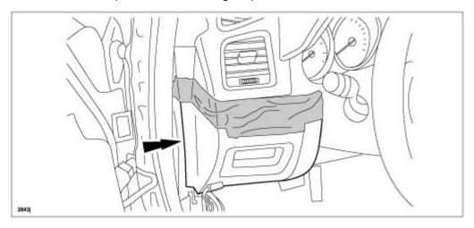
17. Pull the C-15 connector out of the front pillar inside the cabin.
