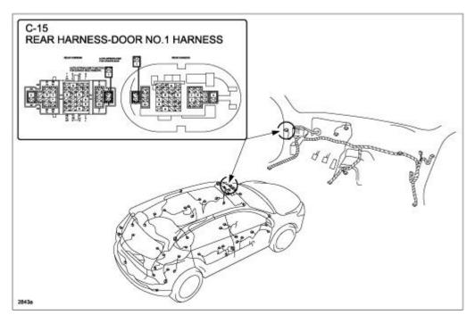
The symptoms listed above may be caused by corrosion of the C-15 connector terminals due to water intrusion through the front door. In low ambient temperatures, the door harness hardens. If the door is fully opened, it may create a gap between the door and the door harness grommet, which may allow water to enter through the gap.
