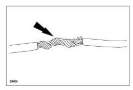
26. Solder the twisted wires together, spreading the solder out across the entire twisted wires.
