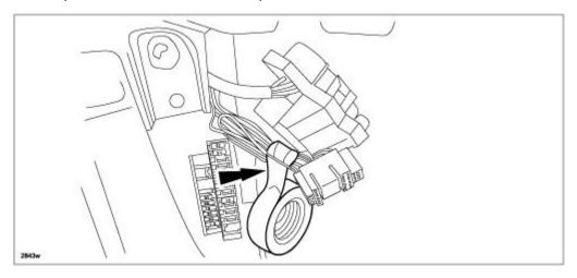
32. Install the protector tube as shown below, then secure both ends with electrical tape.
