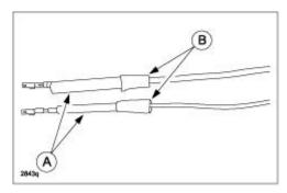
25. Connect the wires from the vehicle side and the wires from the short cord kit by twisting them together.
