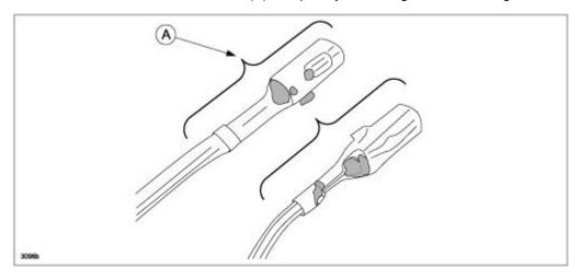
29. Install the repaired terminals into the connector.
