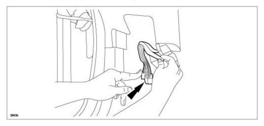
18. Remove the insulation and protector tube for the rear harness to the extent shown below.
