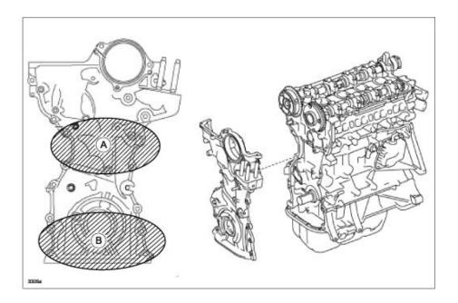
This may be caused by oil escaping from a fine clearance created at the sealant applied to joint (A) between the cylinder block (B) and head (C) when the engine was pressurized during leak testing on the engine assembly line.
