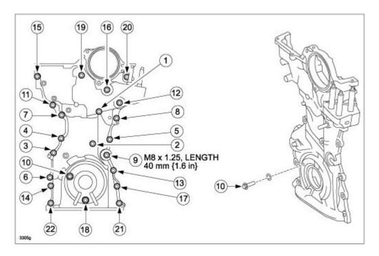
Tightening torque:20-26 N•m {2.1-2.6 kgf•m, 15-19 ft•lbf}
