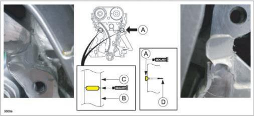
7. Install the engine front cover to the engine.
