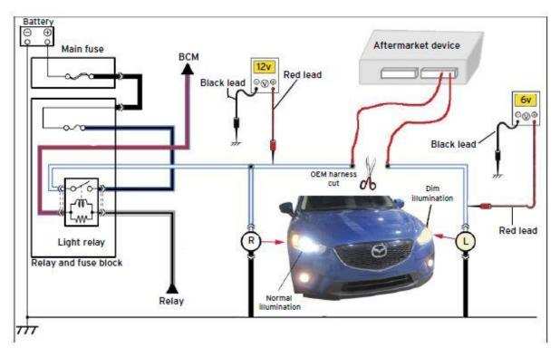
Below is an example of a dim headlight. The aftermarket device changed the headlight circuit resistance, causing a dim headlight.
