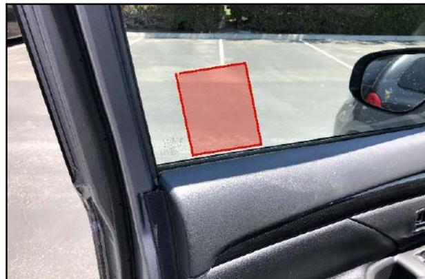
3. Apply label as shown. Label should be parallel to the bottom of the window (@ 5 mm above the rubber) and not cover any part of the DOT information etched into the glass.
