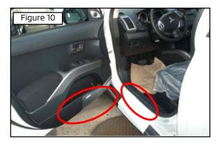
For certain models, the driver entry area is protected by a <u>clear</u> RAP-film placed on the scuff plate and/or lower door area. This is to protect the area from damage while the vehicle is available for viewing by customers or in dealer storage, improving Initial Quality Survey (IQS) scores. The Outlander is protected in both areas while some models are protected on the lower door only. **THIS AREA SHOULD REMAIN PROTECTED BY THE**
