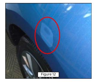
NOTE: If there is still discoloration or blotching or a "milky" color on the paint surface after RAP-Film removal and cleaning (as shown in Figure 12), <u>DO NOT REPAINT THE VEHICLE</u>. Submit a PRC entry with photos for DPSM review, then send the vehicle to a body shop that can use an ultraviolet heat lamp to eliminate milky color spots.
