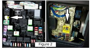
During shipping of Mitsubishi vehicles, dark current is minimized by not connecting the IOD connector. It is positioned in the disconnected position (pulled up) and must be connected by pressing it down for the affected circuits to be completed.
