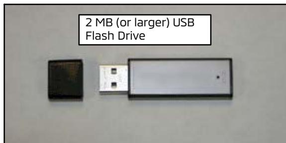
A USB version 2.0 standard flash drive (thumb drive) with a **minimum capacity of 2.0 MB**, formatted to FAT32 is required for this procedure. Formatting to FAT32 will erase all data from the flash drive. The flash drive must have no other files or folders saved to it.
