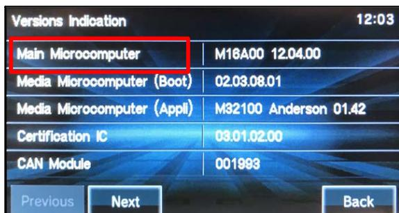
a. On the Versions Indication screen, press and hold "Main Microcomputer" for about 4 seconds, until the Loading Program screen appears.
