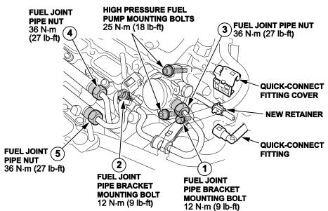
23. Tighten the fuel joint pipe bracket mounting bolts and the fuel joint pipe nuts to the specified torque in the numbered sequence shown.
