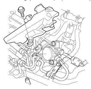
$\ensuremath{\mathbf{27}}.$  Install the intake base and intake manifold.
