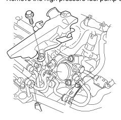
5. Remove the quick-connect fitting cover.
