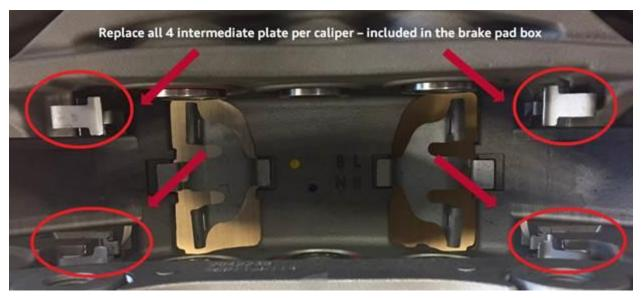
Figure 6. Replace all 4 intermediate plates.
