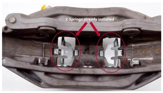
Figure 2. Spring configuration, after installation.
