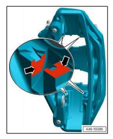
Figure 4. Clean contact surfaces and then coat with lithium grease.
