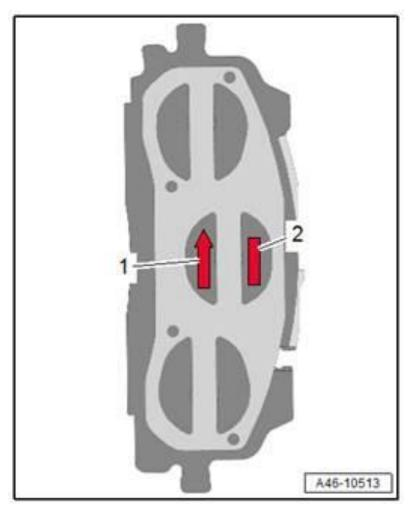
Figure 5. Correct installation positioning for the brake pad.
