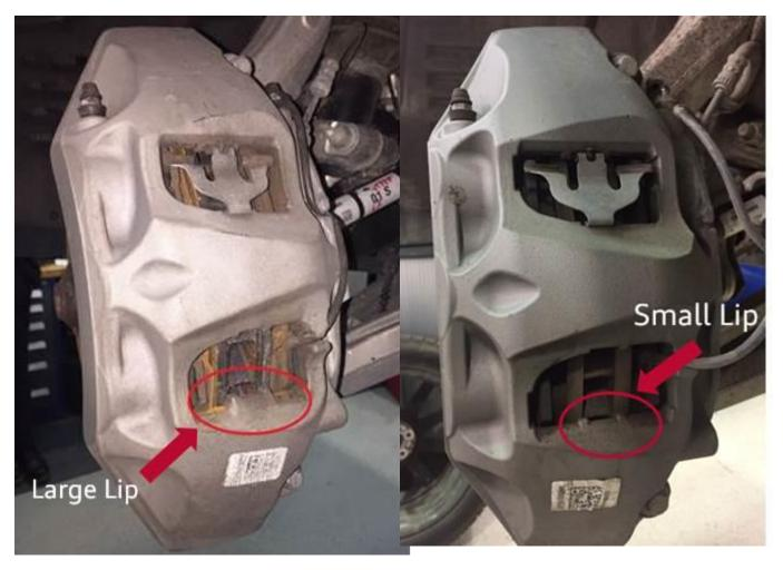
Figure 1. Caliper casting lip configurations.
