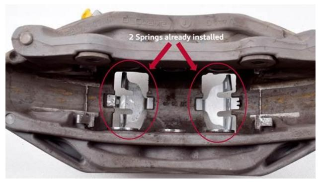
Figure 2. Spring configuration, after installation.
