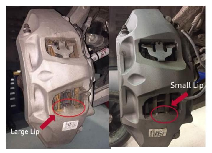
Figure 1. Caliper casting lip configurations.
