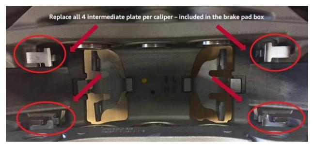
Figure 6. Replace all 4 intermediate plates.
