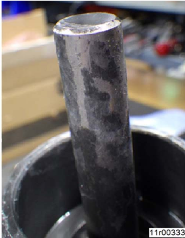
Figure 4 Normal DEF Dosing Valve Inlet Screen
