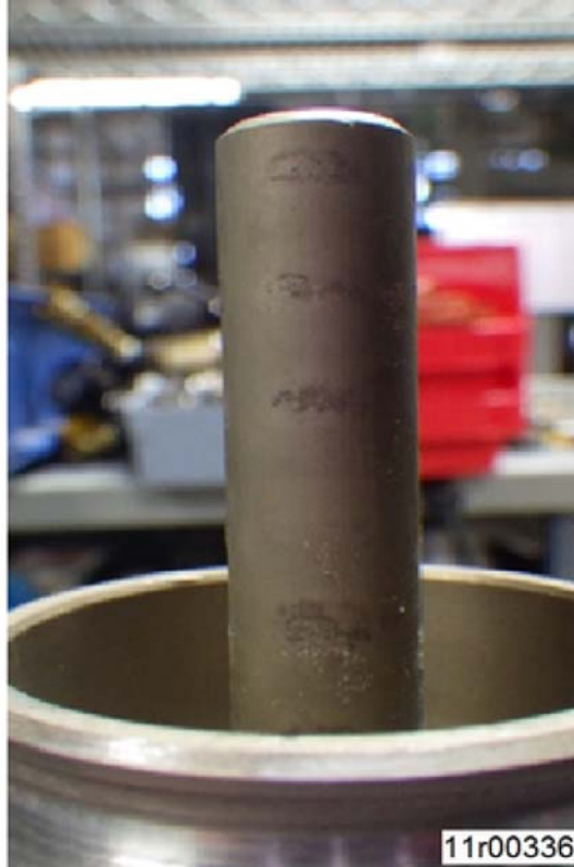
Figure 6 Normal DEF Pump Module Heating Element Discoloration
