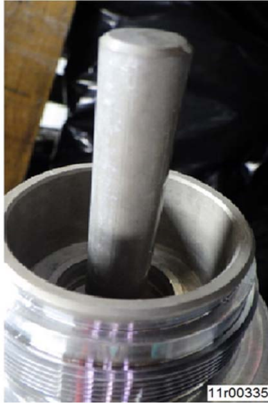
Figure 6 Normal DEF Pump Module Heating Element Discoloration
