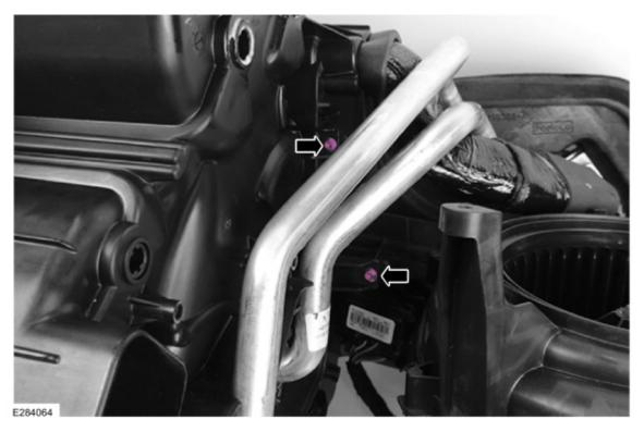
**10.** Remove the 3 climate control housing perimeter fasteners. (Figure 9) Figure 9
