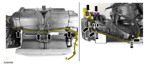
**4.** If equipped with dual zone climate control, disconnect the passenger blend door actuator electrical connector and remove the 3 upper plenum housing to blower motor fasteners. (Figure 3)
