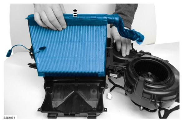
**17.** Install the new evaporator core. Push down on the evaporator core firmly to make sure it is fully seated in the climate control housing. (Figure 16)
