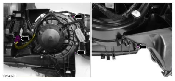
**5.** Remove the 4 upper plenum housing to blower motor fasteners. (Figure 4) Figure 4
