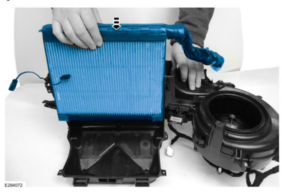
**18.** The new evaporator core may require a minor adjustment to the lines in order to fit properly in the climate control housing. (Figure 17)
