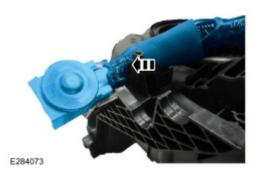
**19.** Install the evaporator temperature sensor wiring seal into the slot in the climate control housing. (Figure 18) Figure 18
