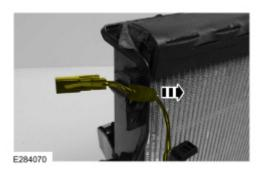
**16.** Remove the evaporator core from the climate control housing. (Figure 15) Figure 15
