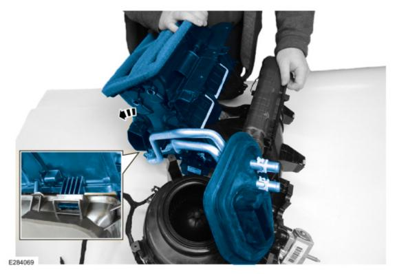
**15.** Remove the evaporator temperature sensor wiring seal from the slot in the climate control housing. (Figure 14) Figure 14
