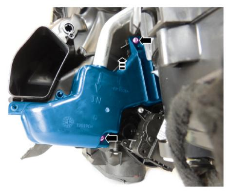
**9.** Remove the 2 climate control housing perimeter fasteners. (Figure 8) Figure 8
