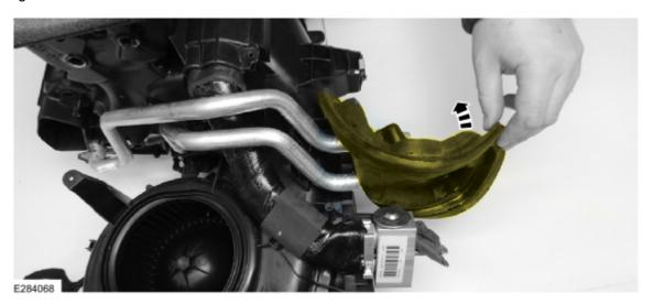
**14.** Remove the plenum chamber and heater core as an assembly from the climate control core housing. (Figure 13) Figure 13
