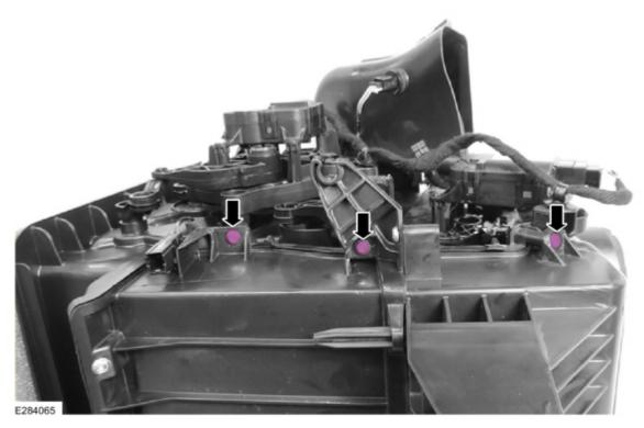
**11.** Remove the 4 climate control housing lower perimeter fasteners. (Figure 10) Figure 10
