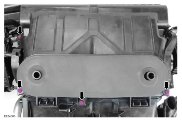
**12.** Remove the 4 climate control assembly perimeter fasteners. (Figure 11) Figure 11
