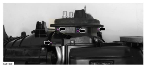
**6.** Position the climate control housing to bulkhead insulator aside and remove the upper plenum housing from the climate control housing. (Figure 5)
