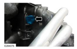
**34.** Remove the old climate control housing assembly foam isolator and apply the new foam isolator. (Figure 21) Figure 21
