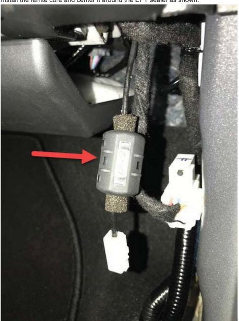
5. Wrap the remaining EPT sealer around the Ferrite Core to secure it in place, and connect the tuner feed harness connector.
