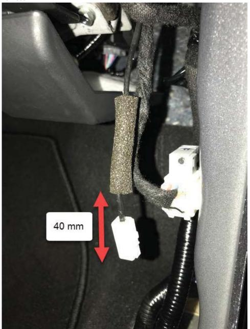
4. Install the ferrite core and center it around the EPT sealer as shown.
