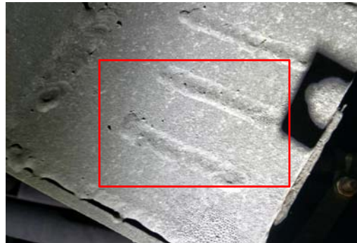
Good Weld: Completely filling slot
