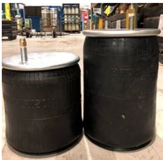
Ex: Uninflated height difference of C-20127 Air Springs
