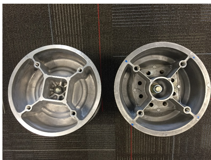
Ex: Piston difference of B-4771 Air Springs
