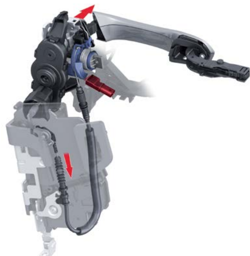
Exterior door operation via a Bowden cable
