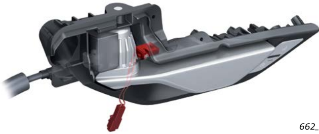
Interior door handle in the rest state
