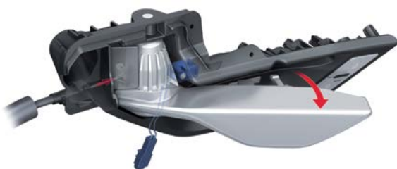
Interior door operation via a Bowden cable
