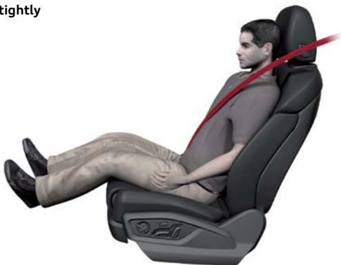
Seat belt on "thick" clothing (greater belt slack)
