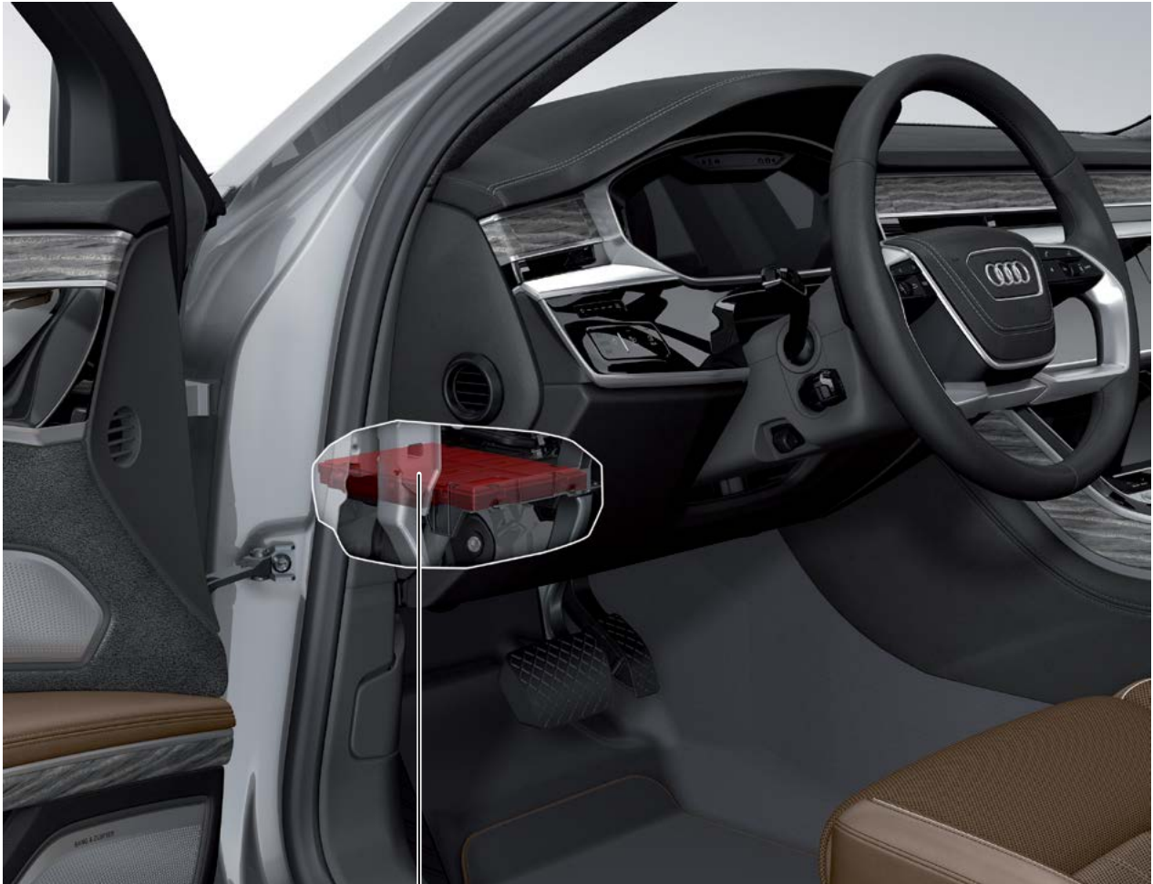
Vehicle Electrical System Control Module J519
