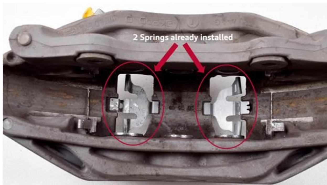
Figure 2. Spring configuration, after installation.
