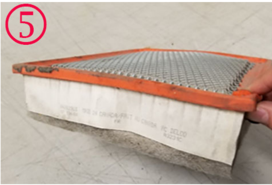
Example of Filter – Early Collapse (Picture 5)
