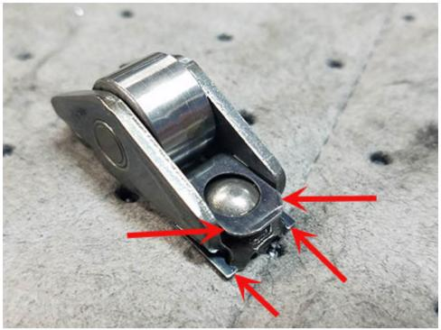
c) If soft , spongy, or damaged SHLAs or rockers are found on either the intake or exhaust side of any cylinder it will be necessary to replace all the affected cylinder SHLAs or rockers and retest.
