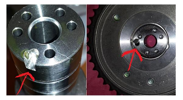
4) If any broken parts are found during inspection replace all damaged parts. It will also be necessary to replace the AFM OCV in the camshaft cover for both banks.
