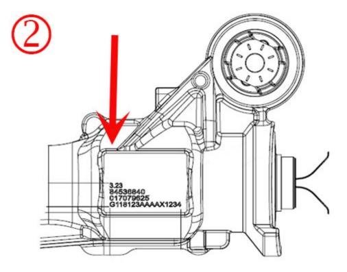
Rear Axle tag location is inboard side of the left hand shock bracket.
