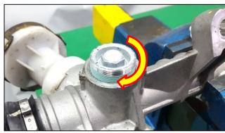
14. Tighten the yoke plug to the torque specification.
