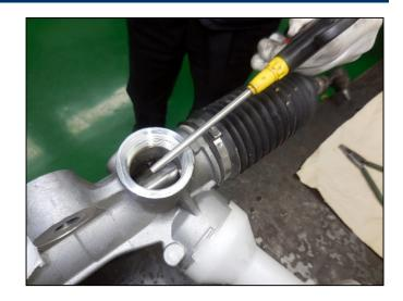
10. Check that the new support yoke o-rings are properly seated.
