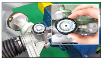
18. While holding the yoke plug with a socket, tighten the lock nut using a torque wrench.
