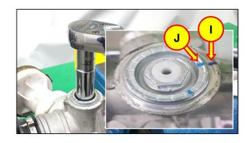
16. Rotate the yoke plug <u>counter-clockwise</u> until the blue yoke plug mark is aligned with the steering rack housing mark created in step 15.
